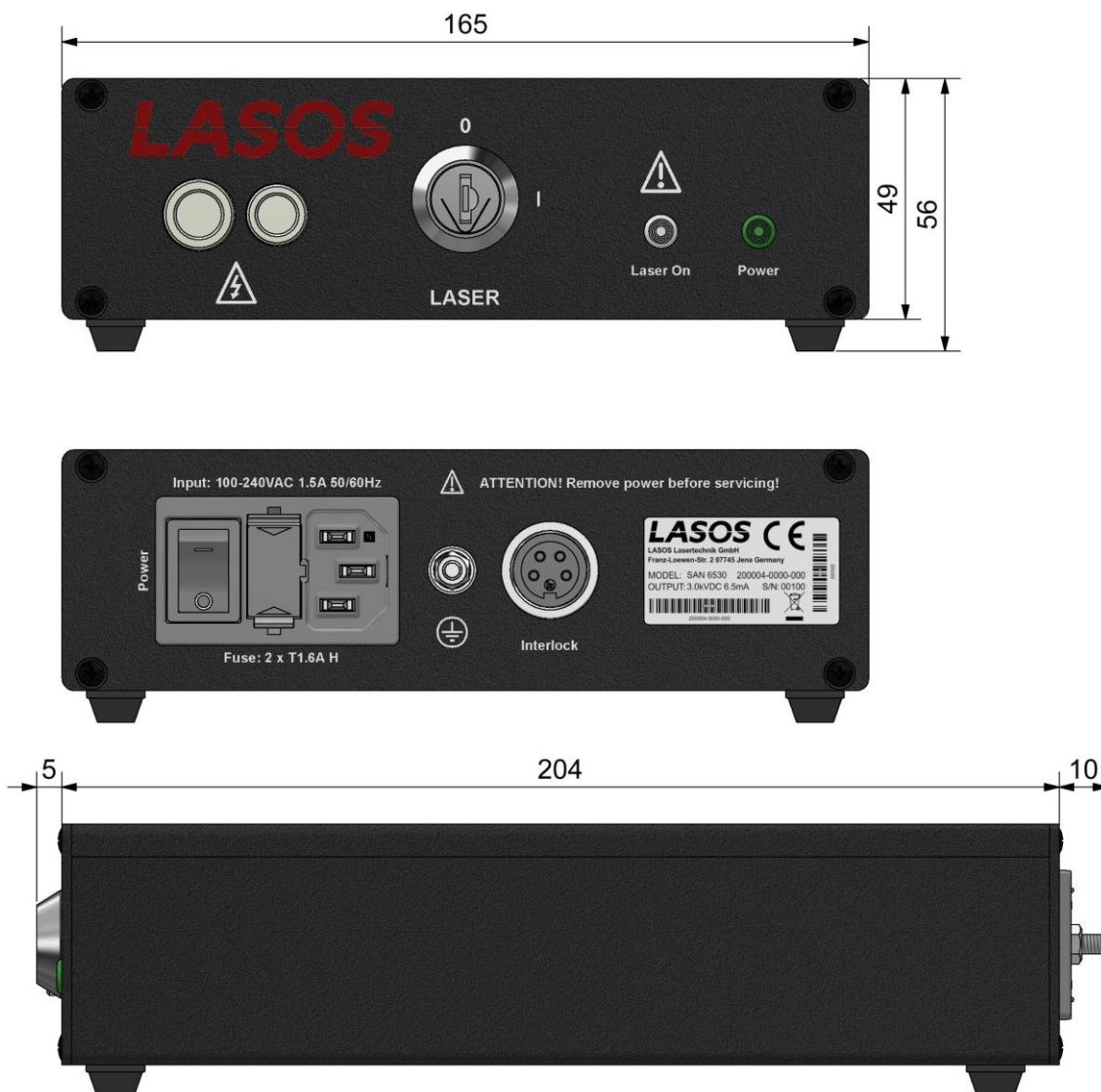
Figure 2 – Dimensions of He-Ne laser laboratory power supply SAN (in mm)
